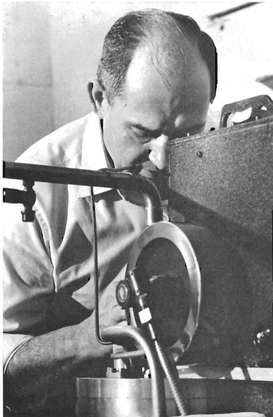
Cryogenic Machinist Gilbert Mulac peers through the viewplate on the helium liquefier to check the level of the liquid.
