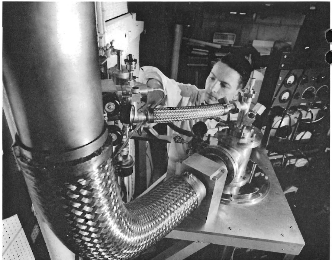
For hypersound experiment, liquid helium must be reduced even lower in temperature. Here, Guernsey assembles apparatus used to pump on liquid helium to reduce its temperature.
