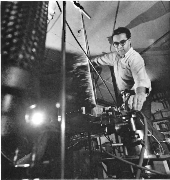
As the cold transfer tube from the container of liquid helium is removed, it freezes the air through which it passes. Note plumes of frozen air near the tube in researcher's right hand.
