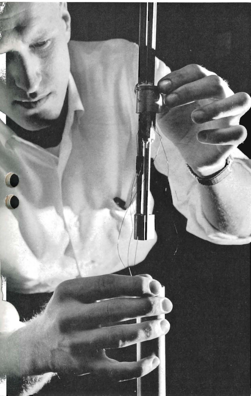
Opfer assembles the sample probe, which will contain the light isotope of helium.
