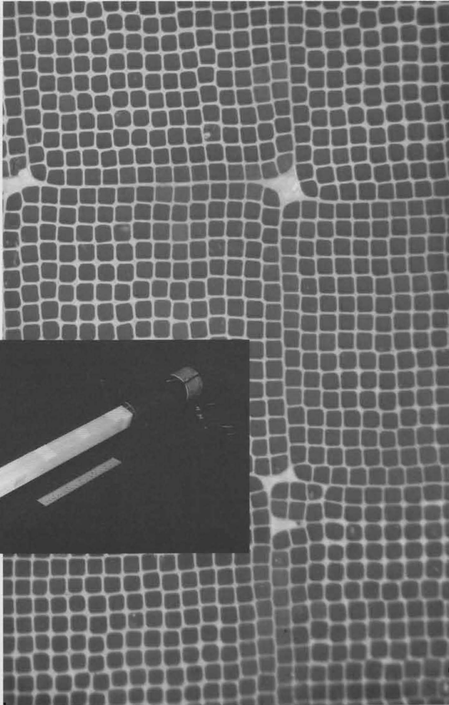
Cosmic eye: a cross-section of SOFIE's scintillating optical fibers. Inset: another view of the optical fiber block.
