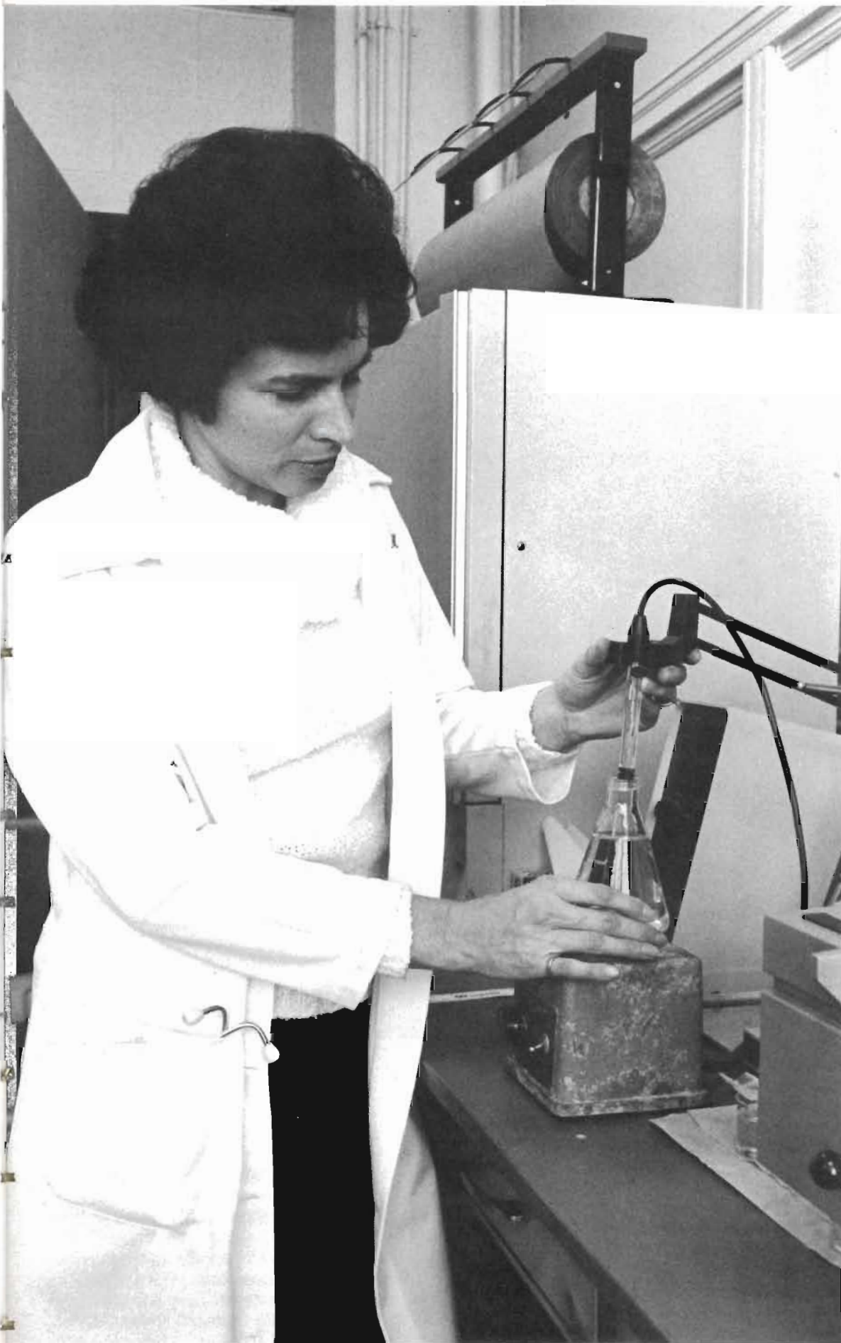
The WUMS Arthritis Center places a great deal of emphasis on both clinical and basic research. Here Hahn uses a pH meter for preparing buffers which are used in her research.
