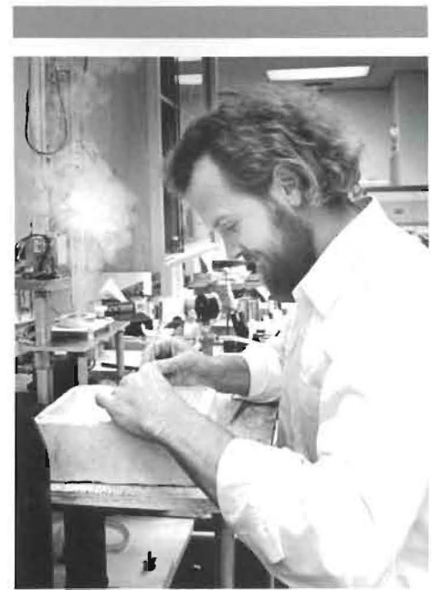
John Heuser, M.D., prepares to freeze-fracture a sample he will view in the electron microscope.
