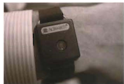
This watch-like device monitors activity and illumination levels for later download to a computer.
